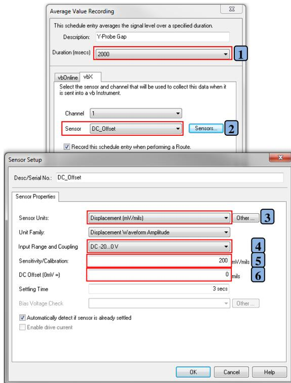
**Figure 4: Gap Voltage and Thrust Position Measurement Configuration**
