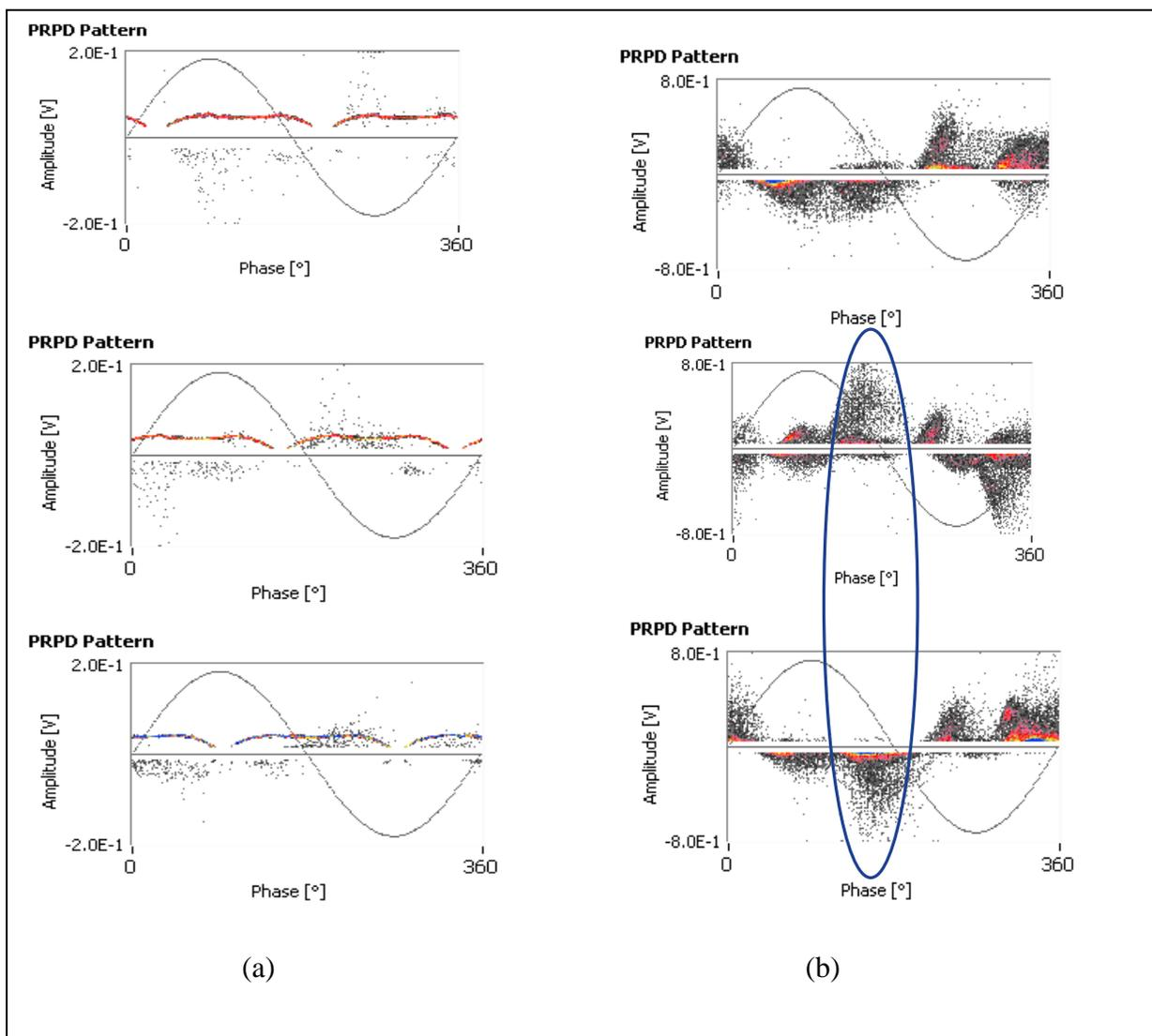
Figure 11. Partial discharge activity (a) before the accelerated insulation aging test (b) just before the motor failed at the end of the accelerated aging test.
